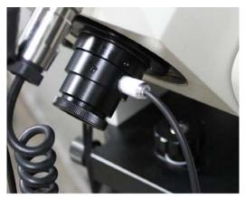
Figure 12. Connect the illumination LED to Polar Scope
