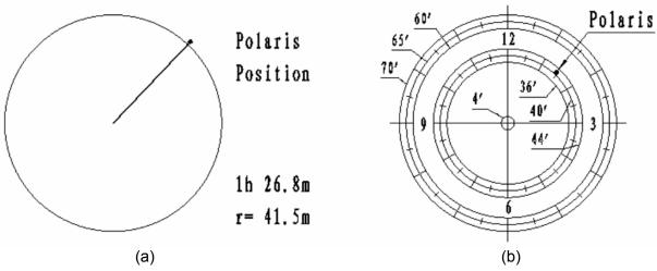
Figure 13. Polaris displayed on 8406 hand controller (a) and Polaris located on Polar scope dial
