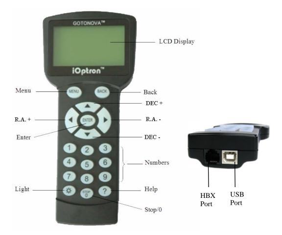
Figure 19. GoToNova 8406 hand controller
