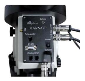
Figure 6. Ports on iEQ75-GT<sup>™</sup> control box
