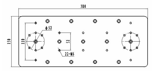
Figure 14. The mounting-hole distribution on the Mount Plate
